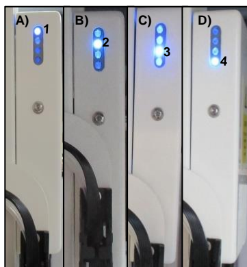
Fig. 6: Four channels of the pressure monitoring system. The blue LED is switched on if the corresponding sample position of the pipetting block is blocked.
